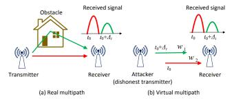
Figure 1: Creating a virtual multipath similar to the real multipath propagation.
