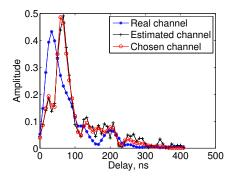
Figure 3: The channel impulse response  $h_r$  estimated at the receiver.
